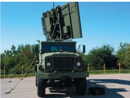
Rapid Antenna Operational Deployment on Single 5-ton Truck
