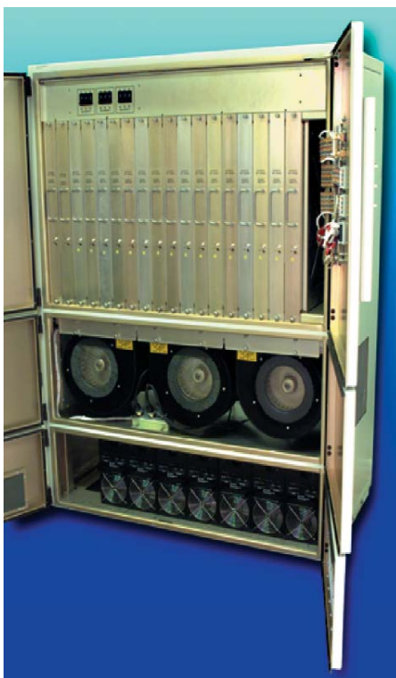
AN/TPS-78 Solid-State Transmitter Incorporates Redundancy Throughout
