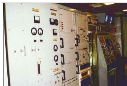
The AN/MPQ-T3A Universal AAA/SAM Threat Radar Simulator (above) is configured in a 12-meter long, fifth-wheel type trailer complete with Control/Operator Consoles (left).
