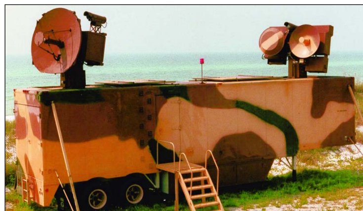
The AN/MPQ-T3A Universal AAA/SAM Threat Radar Simulator (above) is configured in a 12-meter long, fifth-wheel type trailer complete with Control/Operator Consoles (left).
