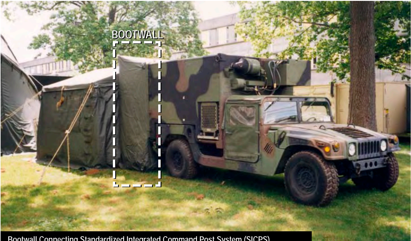
Bootwall Connecting Standardized Integrated Command Post System (SICPS) Rigid Wall Shelter to Modular Command Post System (MCPS) Tent (Army)
