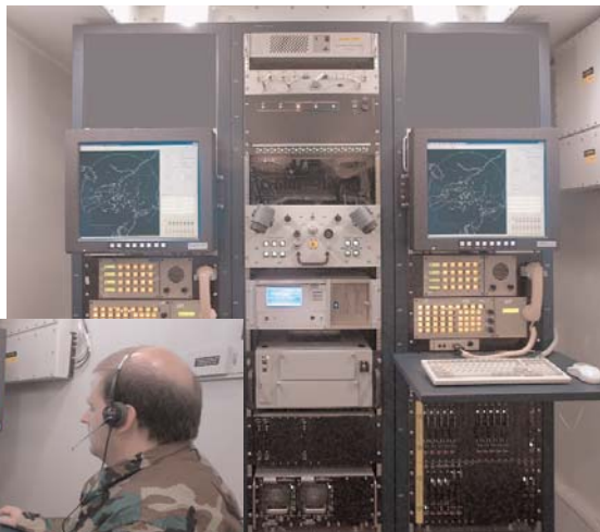
The AN/TPS-77's PMFL system continually monitors the radar status and reports system status to remote maintenance centers.
